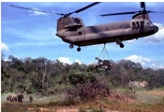
The CH-47 Chinook is a multipurpose helicopter that was often used to sling load heavy weapons, cargo, fuel in rubber tanks, and all sorts of military equipment. Photo courtesy of the author.
