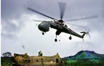
A badly damaged Chinook (on the ground) is recovered by a First Air Cav CH-53 Flying Crane. The Chinook was repaired and returned to service. Photo courtesy of the author.
